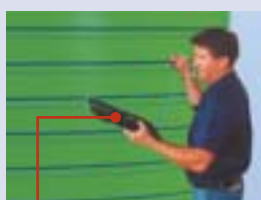
Ultra-sounding of tanks for additional quality control
